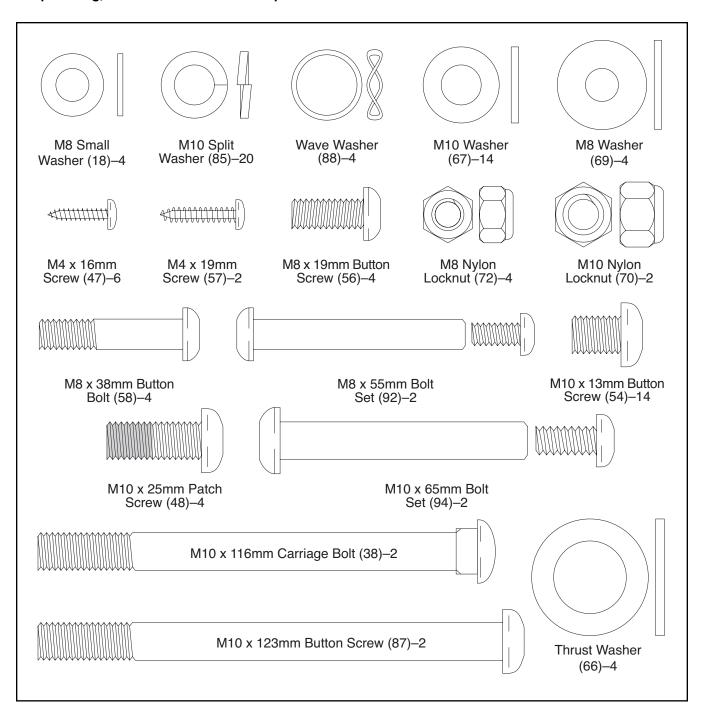
Attach the Stabilizer (8) to the Frame (1) with two M10 x 116mm Carriage Bolts (38) and two M10 Nylon Locknuts (70).
